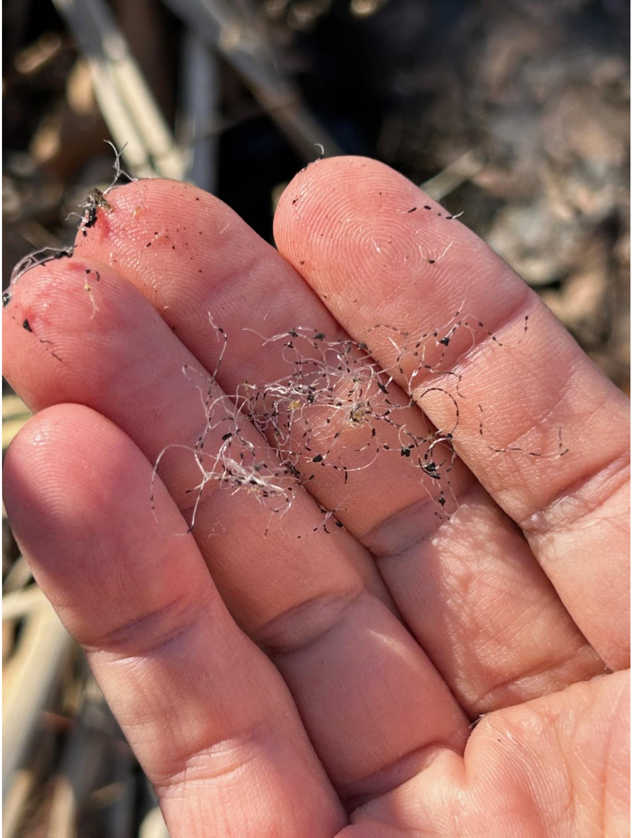
Loose plastic fibers and fragments are easily pulled from islands, indicating brittleness of plastic
